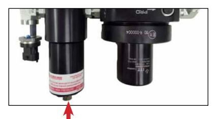
NOTE: For the 2018 model year, the bleeder valve plug is located on the coalescing filter.
