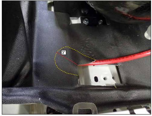
Modify mat to allow high pressure hose to run through.
