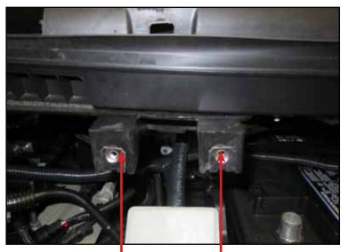
Remove these two tabs. Make a clean cut and flush with the plastic panel. Note: Picture displayed is for the driver side, this must ONLY be done for the passenger side. **Do not touch the driver side tabs.**
